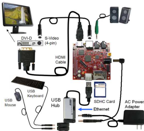
Figure 6: cables and connection diagram for Beagleboard
