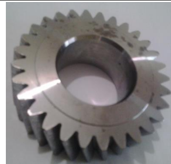
Fig. 5. Showing gear and involute generated through program
